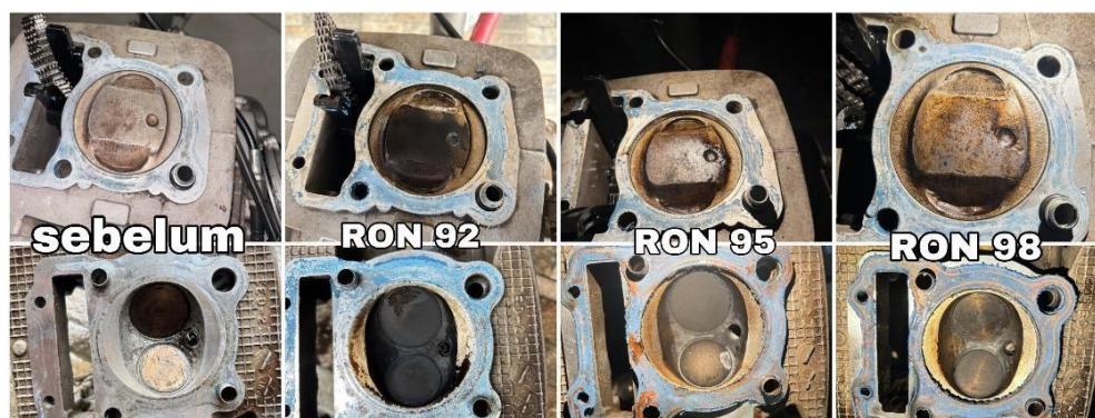
Figure 3. Combustion Chamber Before and After Testing
