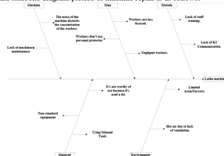
Figure 2 Fishbone repairing lathe machine
