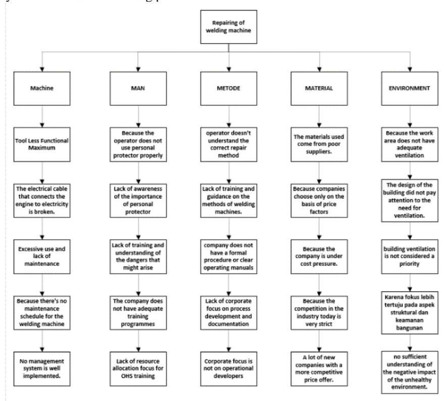
Figure 6 Rca operating welding machine
