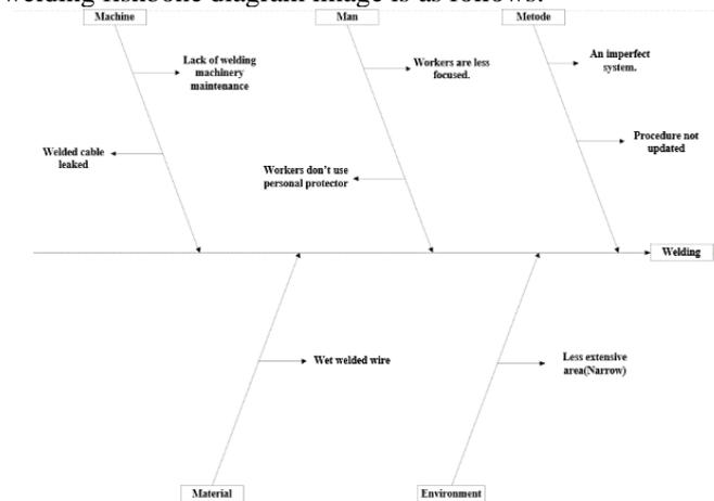
Figure 3 Fishbone welding machine
