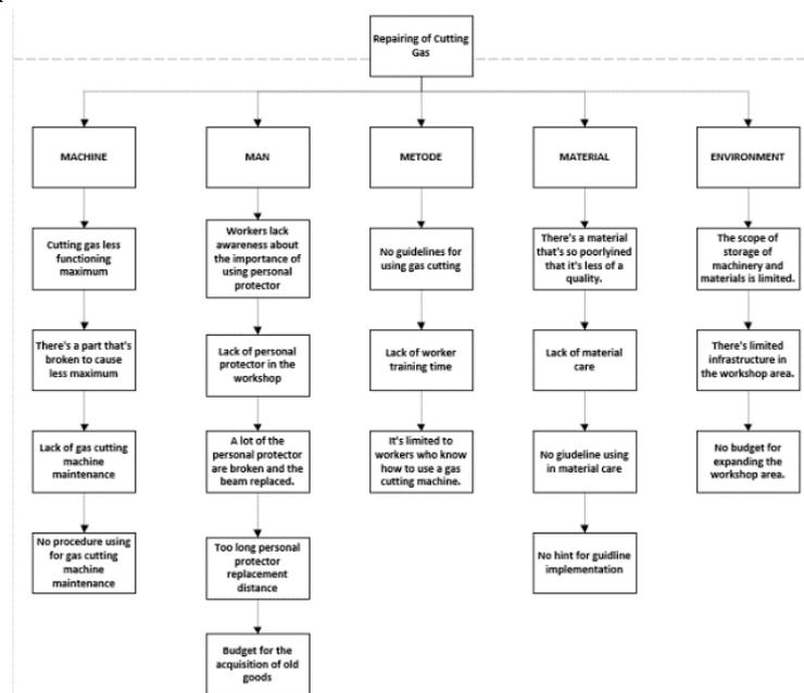
Figure 7 Rca operating cutting gas
