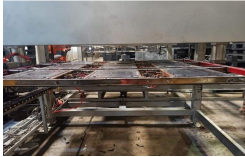
Figure 7. Model Hitter Welding Pallet Type HDX1210R Size 1200 x 1000 mm (Before Improve)
