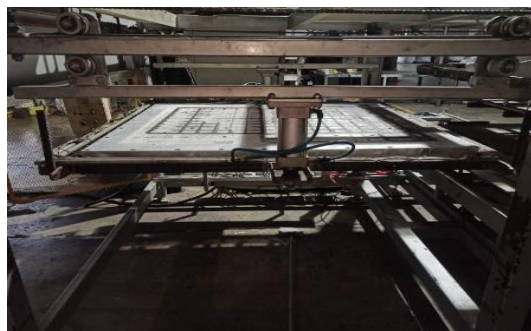
Figure 9. Model Hitter Welding Pallet Type HDX1210R and HD1107 Size 1300 x 1300 mm (After Improvement)
