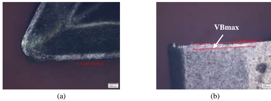
Figure 6. Tool wear of TNMG160404-TF insert. (a) Crater wear, (b) Edge wear
