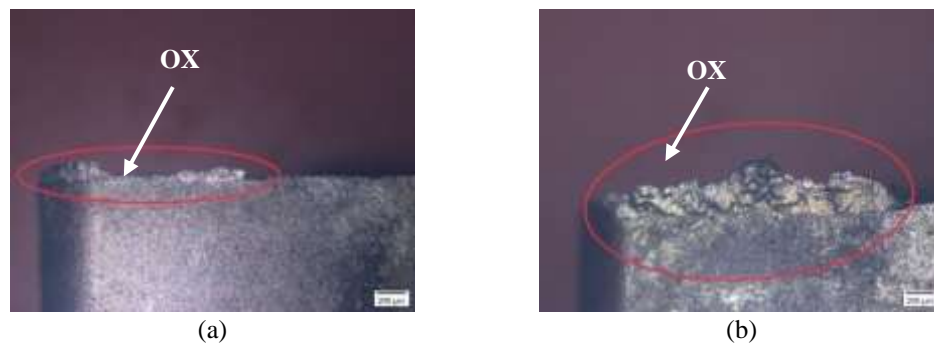
Figure 11. BUE insert TNMG160404-TF. (a) f_1=0.04 mm/put, (b) f_2=0.08 mm/put.
