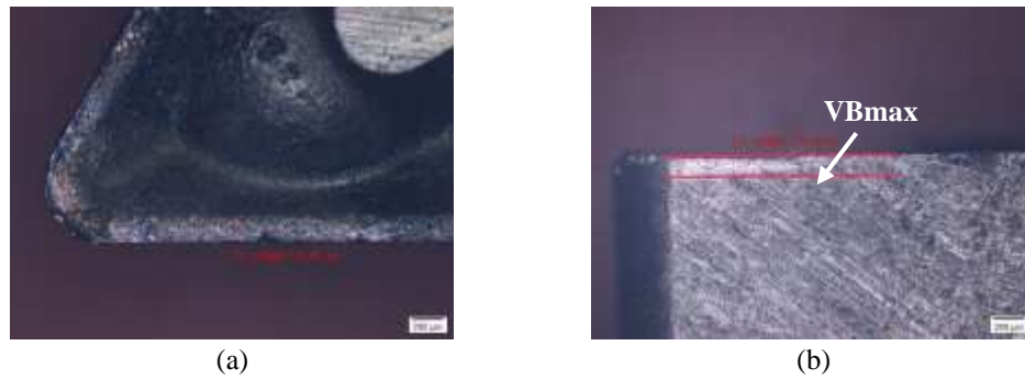
Figure 7. Tool wear of TNMG160404-MA insert. (a) Crater wear, (b) Edge wear.
