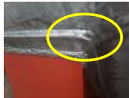
Figure 4 *Undercut Feed drum defects*
