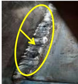
Figure 3 *Porosity Feed drum defects*
