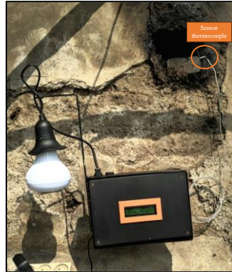
Figure 10. Application of the prototype in a charcoal production furnace
