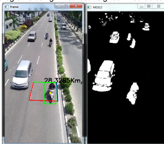
Figure 5. Sample results of testing program using k-nearest neighbor method.
