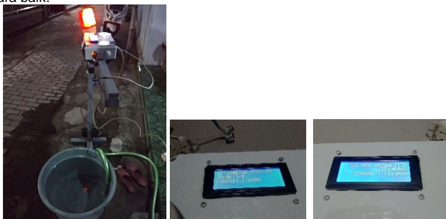
Gambar 8. Proses Uji Coba Monitoring Level Ketinggian Air
