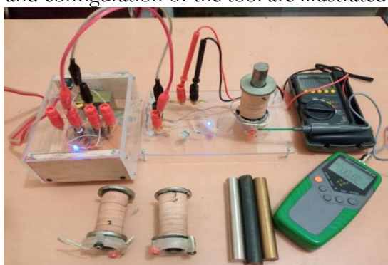
Figure 1. Experimental Tools for Testing The Permeability of Metal Materials
