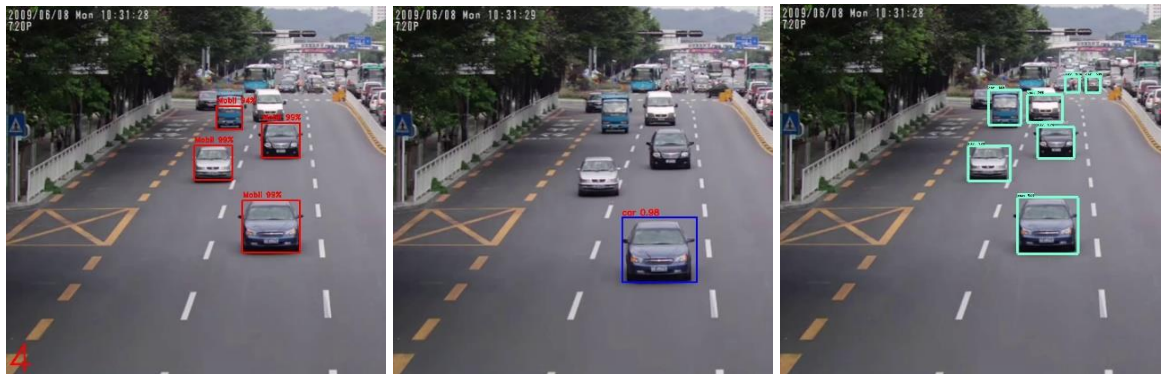
Figure 7. Test Results of the Haar Cascade Classifiers and CNN, YOLO, and SSD methods
